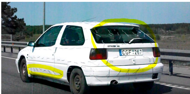
10 pav. Automobilis tiriamas siūliniu metodu Fig. 10. Car is being tuft tested
